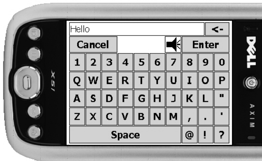
Figure 4. SePA keyboard facilitates data entry via finger taps, which produce typewriter click-like auditory feedback
